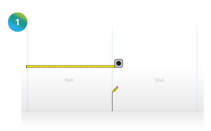
Determine the location of the Hygipods and accurately mark the width of the units onto the wall.
