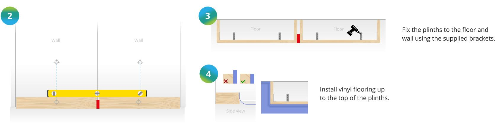
Position the first plinth centred to the first set of markings, then place a 15mm packer between the subsequent plinth.
